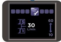
Use the Up and Down buttons to change the setting. Flows > 30 L/min will increment in steps of 5 L/min
