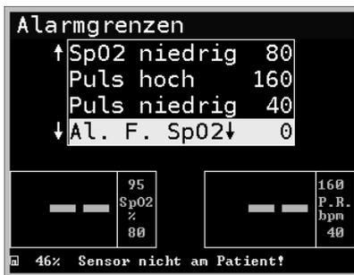
Abb. 49: Alarmfilter SpO<sub>2</sub>
