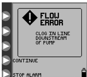
Figure 29. Flow Error screen.
