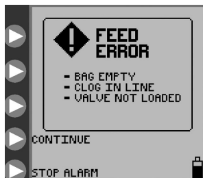
Figure 27. Feed Error screen.
