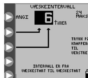
Figur 12C. Stille inn tidsintervall for skylling.
