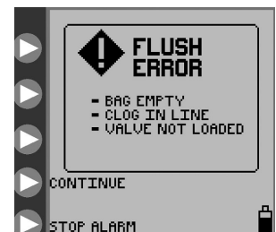
Figure 28. Flush Error screen.
