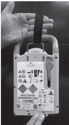
Checking the H300/H850 contents indicator
